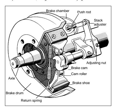
Figure 5-2 S-cam Air Brake
